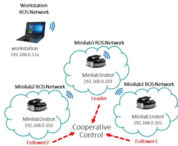
Fig. 8. Multiple robots wireless decentralized communication architecture
